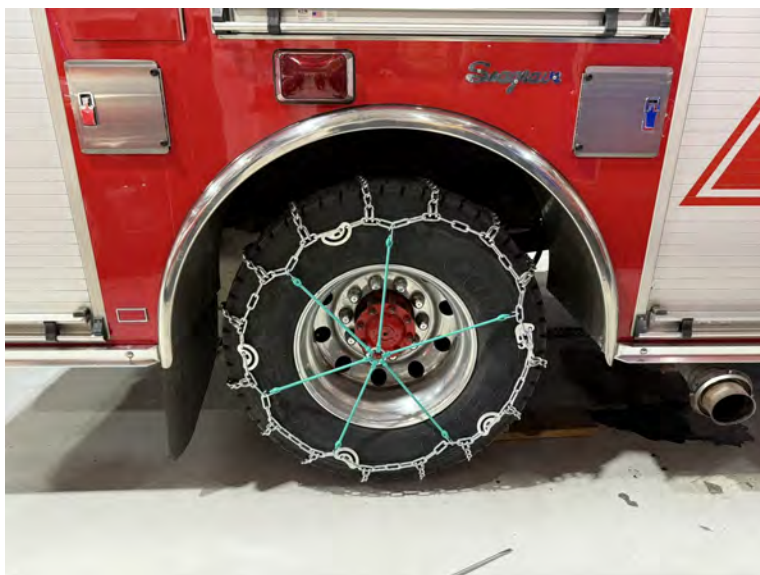
January 2026 — Chains were installed on the trucks to improve traction on snow-covered roads.
